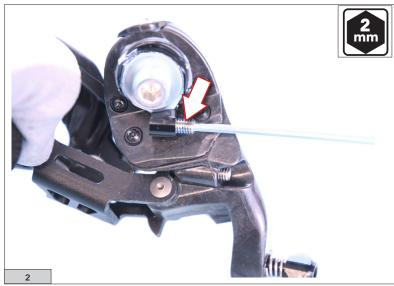
• Use a 2 mm Allen key to install the direct mount rear derailleur positioning screw with joint (Fig. 3).
