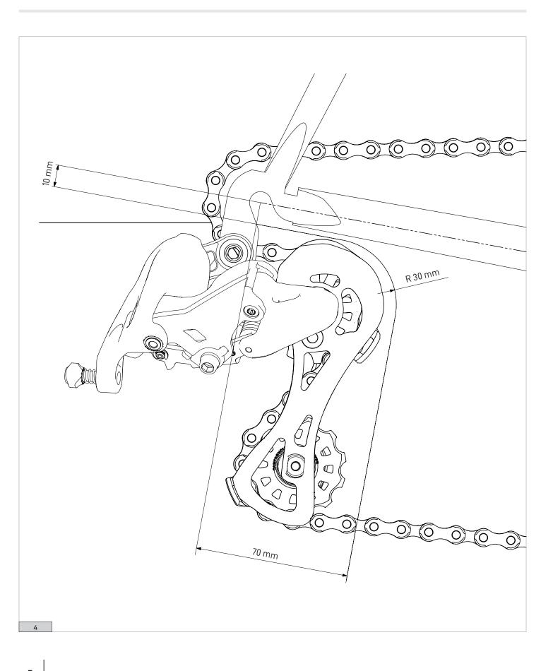
For the first 70 mm between the wheel axle and the bottom bracket, the right chainstay must not fall more than 10 mm inside the direct line between the axle and the centre of the bottom bracket.
