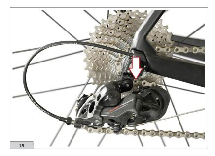
• that there is a correct ascent and descent between the smaller sprocket and the nearby sprocket with the chain positioned on both chainrings.
