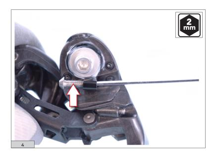
• Use a 2 mm Allen key to install the rear derailleur positioning screw with joint (Fig. 5).
